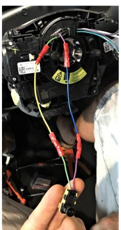
Go ahead crimping the 2 terminals to the wires coming out from the clockspring assembly. BE CAREFULL NOT TO MISMATCH THE WIRE COLORS. If a wire comes out from the clockspring , for example, in green, then the terminal must be crimped to the green wire that goes to the little airbag connector, and so the other one. Some cars does have 2 airbag connectors because of being dual stage airbag. In this case, repeat the procedure on the other connector.
