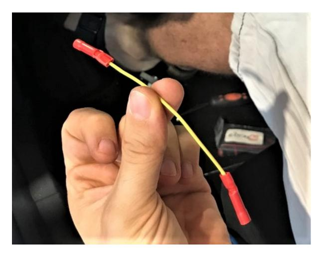
4) Crimp the 2 extensions to the pending wires coming from the airbag connector.
