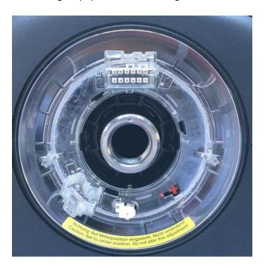
The OEM harness is made by 12 wires gathered in a 6 + 6 pin connector. The provided wire extension is made by a 6+6 pin harness. The connectors are not the same with the secure clicklock, but the pins need a bit of force to match the contacts, and they're not going to disconnect unless you applicate a force which is much more than any dynamic action which may appen during driving.
