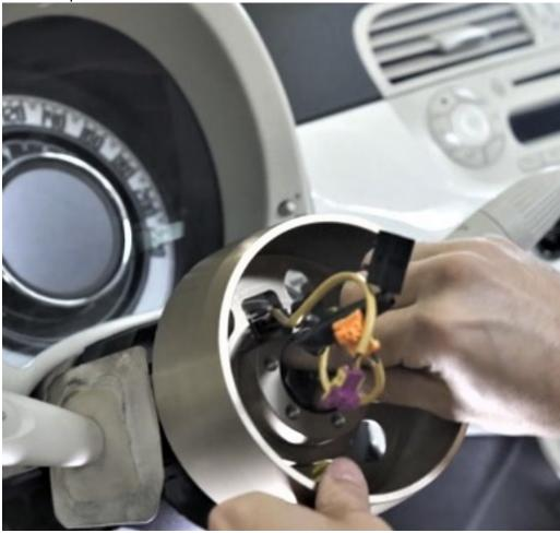
Use the OEM nut to tight the aluminum hub on the steering column at 60 Nm.
