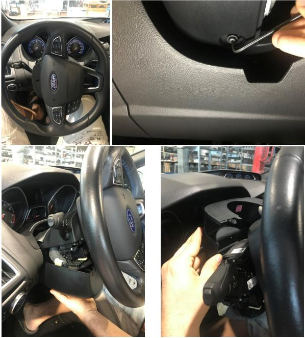
2) Take a flat screwdriver, grind the point to make it concave to better press the springs, and press the 2 springs, 1 at each side. When pressing, the corresponding part of the airnag will pop out a little bit.
