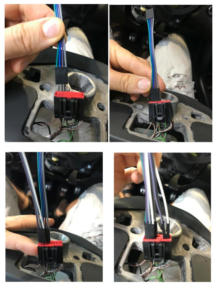
To cut and extend the airbag wires, proceed as follows:
