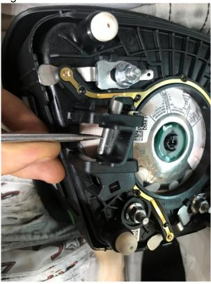
3) After the airbag is out, unplug the connector. Lift the secure lock clip with a flat screwdriver, as shown in the picture. You don't need a lot of force, just be accurate. You need to lift the clip to unplug the connector.
