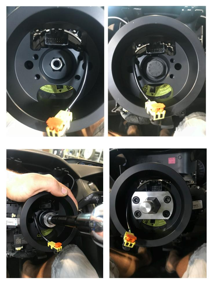
14) Insert the steel part on the aluminium part.and tight the M6 bolts at 10 Nm.
