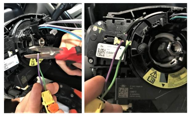
10) Peel the wires at each terminal generated after the cut
