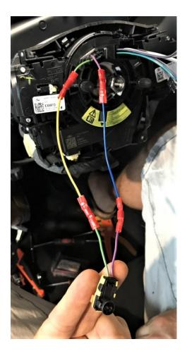
In the picture at the left side you're going to see the final result. You can now complete the steering wheel spacer installation. 13)Insert the aluminium part in the shaft. Make the wires go through the slot gently. Tight the central bolt that was holding the steering wheel in place at 60 Nm.
