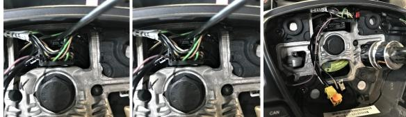
7) Pull the steering wheel out and lay it in a safe and clean place: You will see the same as in the pic below on the right.
