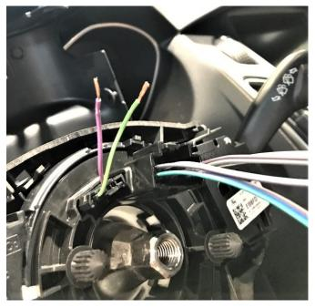
11)Purchase some wire, same AWG of your airbag wires, and cut 2 pieces, same length as the spacer, 5 to 6 cm (2" to 2" ½). Much better if the wires are the same color of your airbag wires. Peel the end of the wires as you did for the car's wires. Crimp 4 x terminals crimp-pipes fittings. You now made your extensions.
