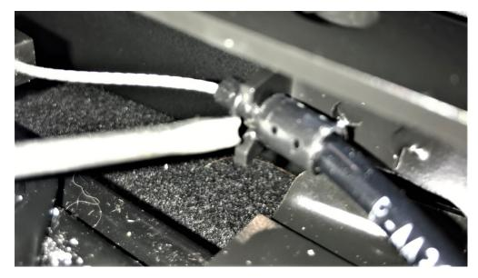
11) No the seat is re-assembled and the 2 brackets in line between each other. Bolt the rails back on the brackets. You will need again to move the rails back and forth to free the holes in which insert the bolts.
