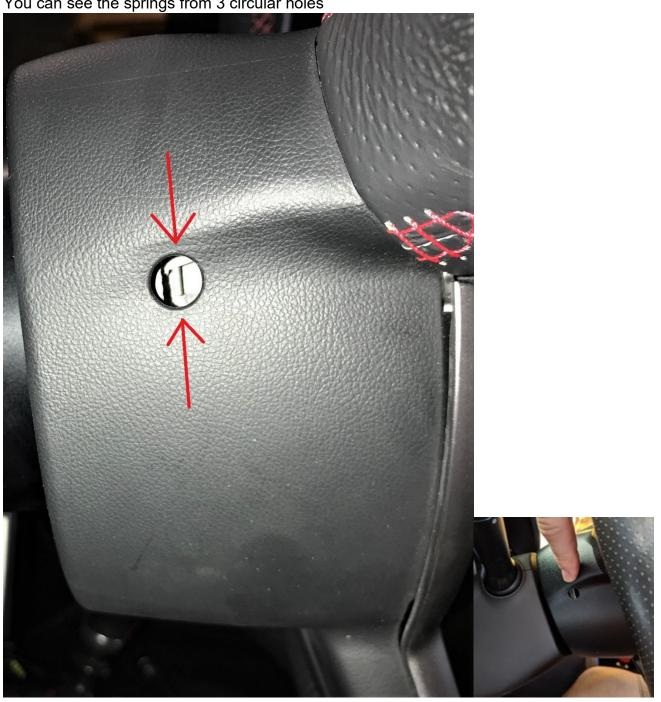
This is how the springs look after you remove the airbag, to help understand how to unclip them.
