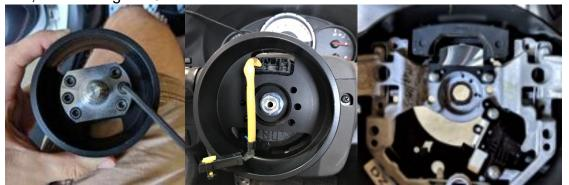
6) Fit the aluminum side of the steering wheel spacer on the steering column, keeping the orientation of the slots horizontal. The little slot must stay up as it is on the steering wheel. The
