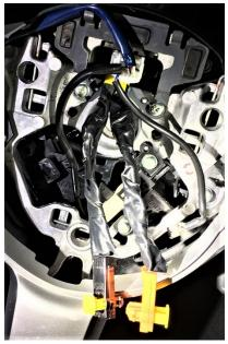
Push the airbag in the steering wheel assembly, making the engagement of the 3 springs which you have touched at the begin. It's a bit more than pressing the horn.
