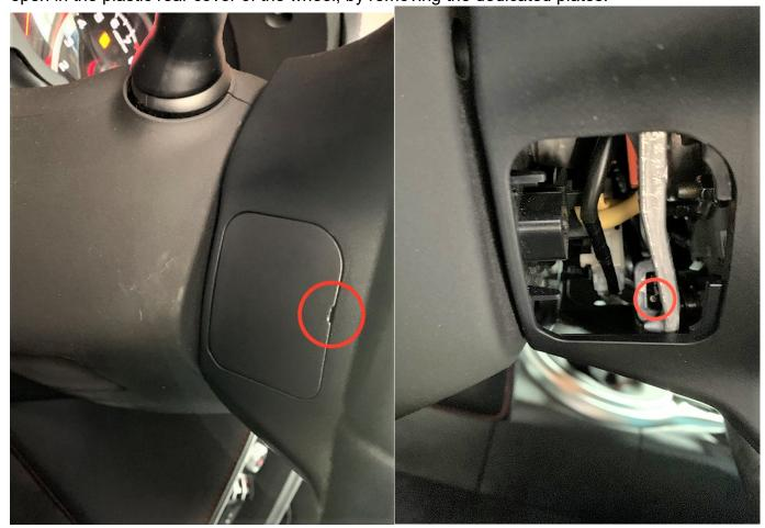
This is how the springs look after you remove the airbag, to help understand how to unclip them.
