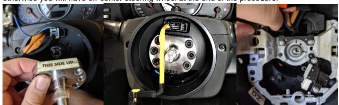
8) Insert the provided harness for the steering wheel commands in the central connector of the clockspring assembly. It has a single way to get in and makes a reassuring "click" when is in. You will connect the other side to the OEM connector which comes from the steering wheel in a second moment.
