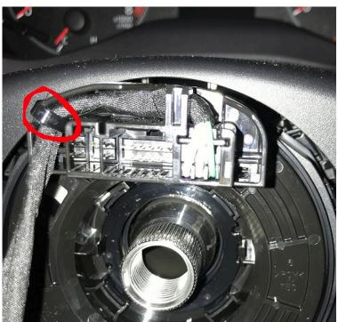
6) Insert the provided harness in the corresponding central connector, to extend the steering wheel buttons wires. There is only 1 orientation possible, and it makes a secure lock "click" once well pressed inside.
