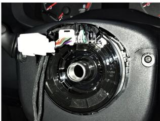
7) Fit the female splined spacer in the steering column. The back side of it has the slots exactly as in the steering wheel. The airbag + steering wheel buttons wires must cross the spacer through the top slot with a flat side. The heated wheel wires, if present, must cross the spacer through the bottom slot without flat sides.
