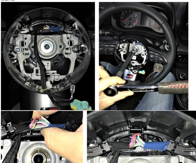
4) At this point, the steering wheel will come out easily, while you pull it out, gently make the airbag wires slide across the slot in the steering wheel, without being pulled in any moment.
