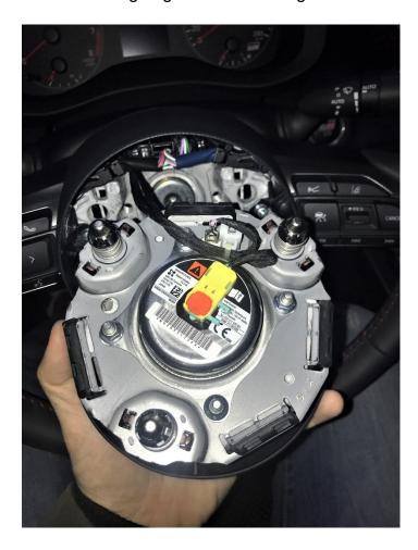
2) To fully separate the airbag from the car, you have to disconnect 3 connectors. 1 for the airbag itself, yellow/orange, another white little connector, and the horn's faston. You will need a little flat screwdriver to lift the secure locks. Start with the airbag wire, lifting the orange secure clip and pulling out the connector as shown in the pictures.
