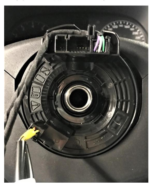
5) Cut the black cable tie on the top left of the clockspring assembly. This is a cheap part, very easy to replace, and pretty useless too. It free up some length on the airbag wires, and helps with the clearance between the spacer and the clockspring, which is very tight in that point. PAY ATTENTION not to cut the airbag wires too, even accidentally, or you will need to replace the expensive clockspring assembly too.
