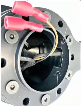
**AGAIN, WARNING**: after you connect the big red/black connector, push GENTLY the black wire in the room inside the black boot. Don't bend it too tight, let it make big radius turns. The harness has some resistances inside that emulates the OEM paddleshift electronic circuit and these resistances are pretty easy to damage if bent. If you push the harness gently inside the collapsible hub's room, it will "live" inside it for long time, but pay attention not to push it roughly.
