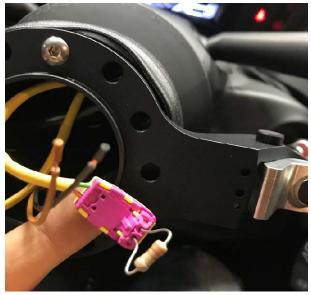
8) Insert the steering wheel in the centering of the frame, and tight the 6 bolts. Connect the 2 fast-ons coming from the kit, to the horn button (not included in the kit). THE END.
